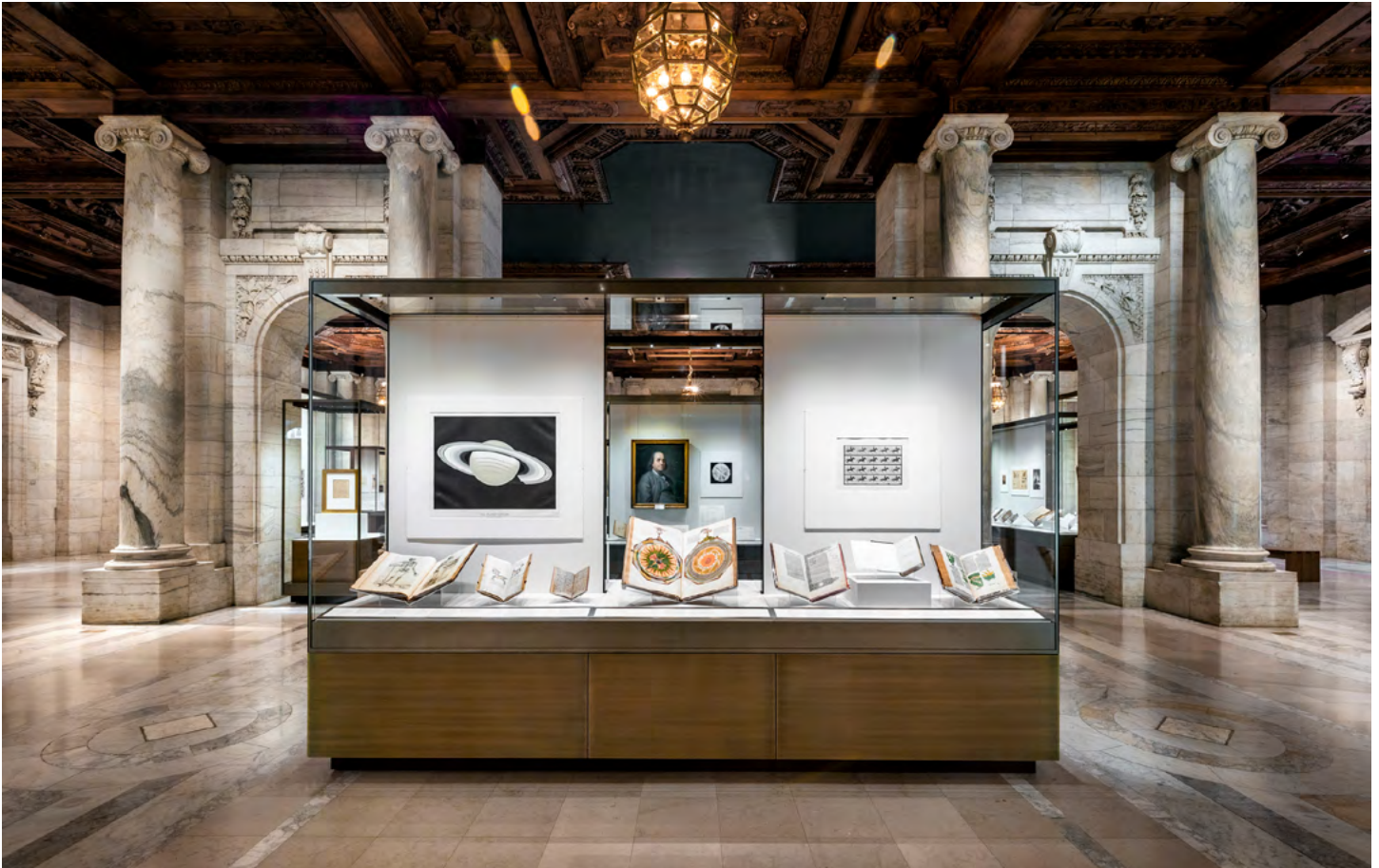
ABOVE: The casework, manufactured by Goppion, is clad in a bronze patina to match Gottesman Hall's existing finishes. BELOW: Cut-throughs in the display walls of the case interiors allow views of other sections of the gallery.
